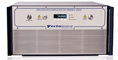
The amplifier can be controlled from either the front panel or remote control via the Ethernet, USB and GPIB interfaces. The digital interface system manages enabling and disabling the amplifier, monitoring power levels, monitoring power supply health, communicating with the control computer and implementing electrical interlocks. The keypad and display interface is used for monitoring amplifier state, power levels, interlock states etc. and for configuration options.
