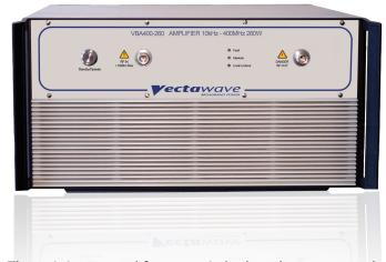
The unit is powered from a switched mode power supply for high efficiency, high power factor and wide voltage range operation. The unit is air-cooled with integral fans, and is protected against faulty cooling by excess temperature sensing. Two safety interlock connectors are provided, one to short for interlock and the other to open circuit. Front panel indicators are provided to indicate over-temperature, standby and operate and rf interlock operation.
