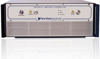
The amplifier operates in class A, the benefits for EMC applications being very low distortion and tolerance of 100% mismatch. Fold-back protection is neither fitted nor needed! This makes it supremely suited for very demanding transducer and test chamber requirements.
